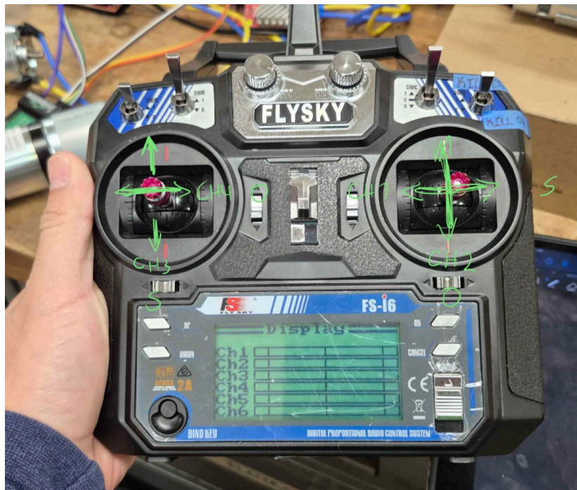
Default joystick → channel mappings from the RC controller to the roboclaw.
