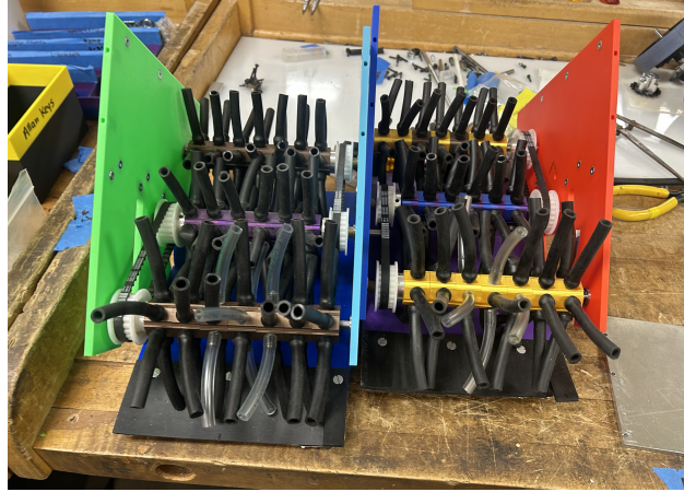
Figure 10: Intake Assembly of Both Robots before Final Assembly
