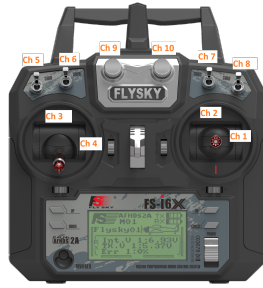
Figure 16: Controller channel configuration
