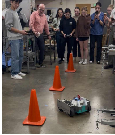
Figure 20: Navigation test for mobility demo with drivetrain prototype
