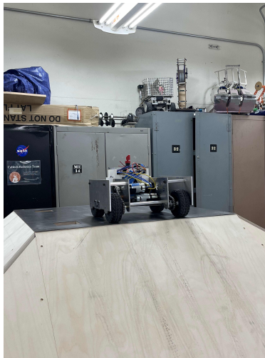
Figure 19: Drivetrain prototype for first drivetrain mobility demo
